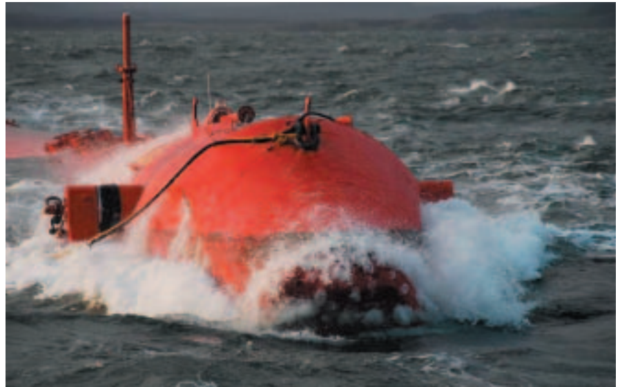
The Pelamis Wave Energy Converter (WEC) [Courtesy: Ocean Power Delivery].
