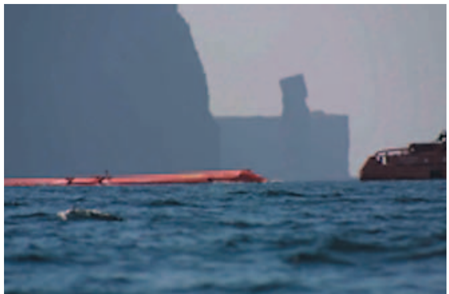
The Pelamis Wave Energy Converter (WEC) [Courtesy: Ocean Power Delivery].
